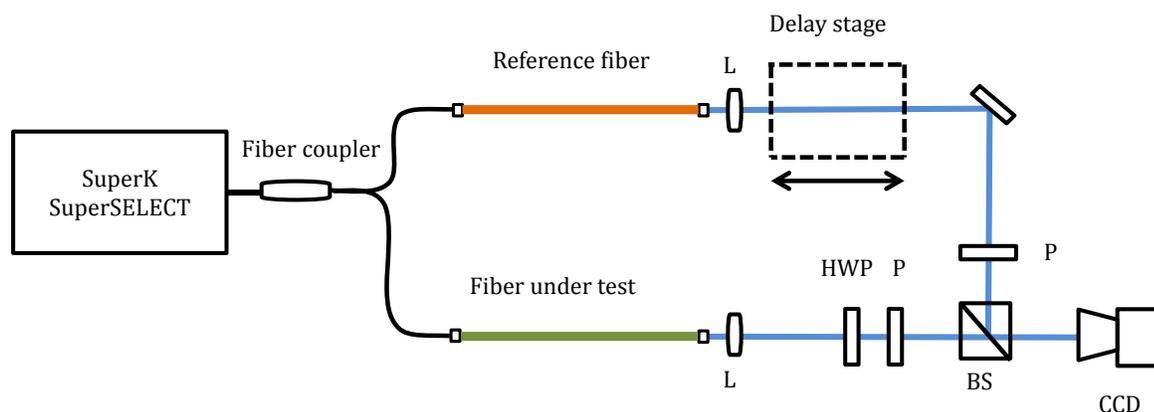
Figure 1. The scheme of the experimental setup for the improved  $C^2$  measurement. Here, *SuperK* and *Super SELECT* are applied in the setup as a light source and a filtering box, PM coupler - polarization maintaining fiber coupler, L - lens, P - linear polarizer, BS - beam splitter.
