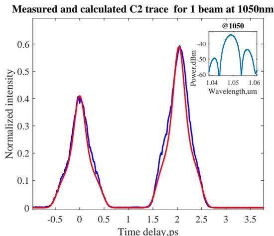
Figure 3. The measured (blue curve) and calculated (red curve)  $C^2$  imaging trace for one channel from *SuperSelect* at the central wavelength at 1050nm. The inset shows the measured spectrum that was implemented in the theoretical calculation and at the measurement.
