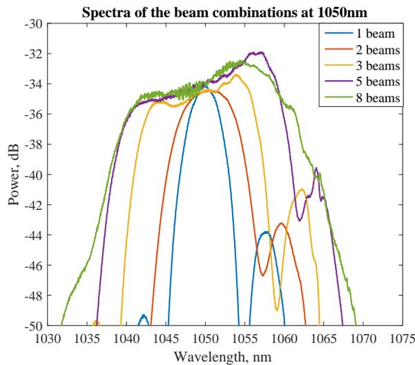
Figure 5. Input spectra merged from 1, 2, 3, 5 and 8 beams.
