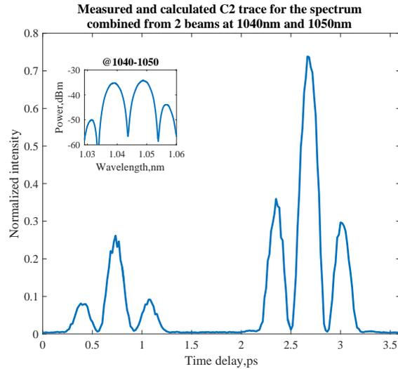
Figure 4. The measured  $C^2$  imaging trace for 2 turned on channel from *SuperSelect* with a separation in wavelengths of 10nm at the central wavelengths of 1040nm and 1050nm. The inset shows the measured spectrum that was used in the theoretical calculation and at the measurement.
