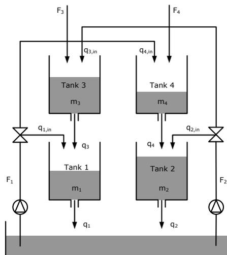
**Figure 1.** Schematic diagram of the modified quadruple tank process
