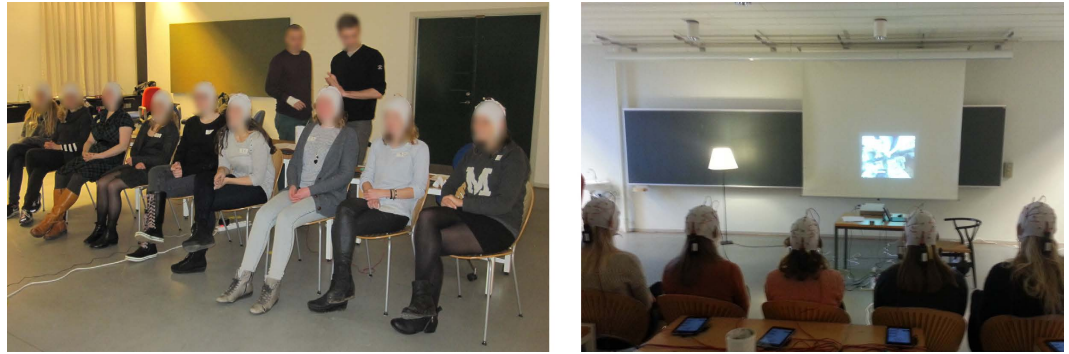
Figure 1. Experimental setup for joint viewings. (Left) 9 subjects were placed on a line to induce a cinematic-like experience. (Right) Subjects seen from the back, watching films projected onto a screen. Tablets recording EEG are resting on the tables behind the subjects. The signal is transmitted wirelessly from each subject.
