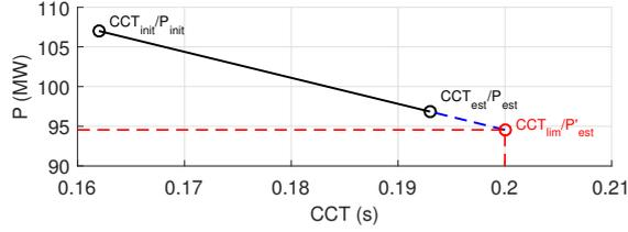
Figure 4: Extrapolation of initial and estimated condition to obtain the next power setpoint  $P'_{est}$ , for which  $CCT'_{est}$  is determined. (Values of the plot are irrelevant, but they are shown for clarity.)
