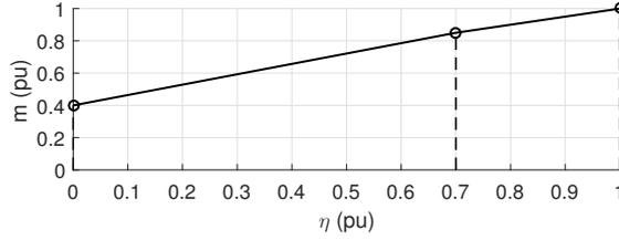
Figure 3: Estimation of the generator's power setpoint
