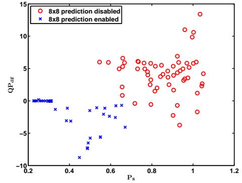
Fig. 7. Detection of 8x8 prediction using the  $QP_{dif}$  (18) and  $P_8$  (19) values.
