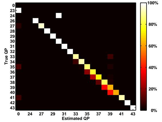
Fig. 4. I-frame  $QP$  confusion matrix for the LIVE database. The estimated  $QP$  is equal to 0 when  $N_{tot}^i < 9, \forall i$ , i.e. we do not have enough data for that frame (which is the case for 2% of the I-frames). For the rest of the estimated  $QP$  values the RMSE is equal to 0.77. (The reason for the apparently large error at original  $QP = 24$  is due to the fact that there is only two frames with this particular  $QP$  in the whole dataset and they are both wrongly estimated.)
