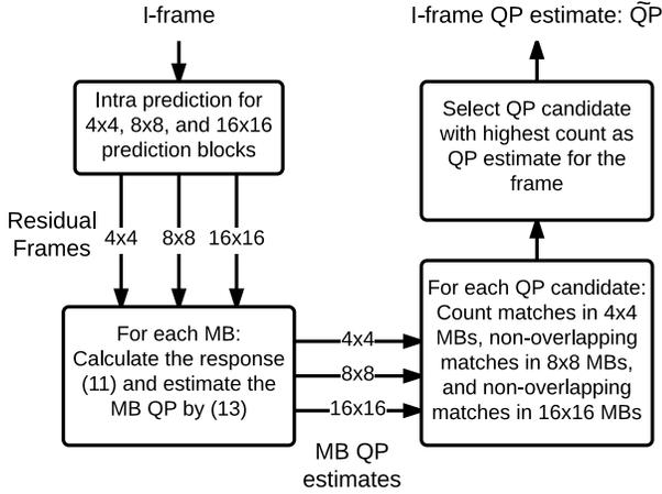
Fig. 3. Block diagram of the I-frame QP estimation
