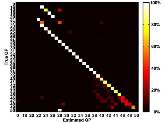
Fig. 5. I-frame  $QP$  confusion matrix for the Lisbon database. The estimated  $QP$  is equal to 0 when  $N_{tot} < 9, \forall i$ , i.e. we do not have enough data for that frame (which is the case for 0.1% of the I-frames). For the rest of the estimated  $QP$  values the RMSE is equal to 2.2. (Since the proposed method only considers  $QP \in [21, \dots, 51]$ , all the original  $QP$  parameters outside this range is wrongly estimated.)
