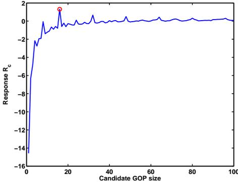
Fig. 6. Illustration of the response  $R_c$  as function of candidate GOP sizes for the "Pedestrian Area" video at highest bitrate from the LIVE database. The value of the true GOP size is marked by a red circle. This value coincides with the input value giving the maximum response  $R_c$  value for this example.
