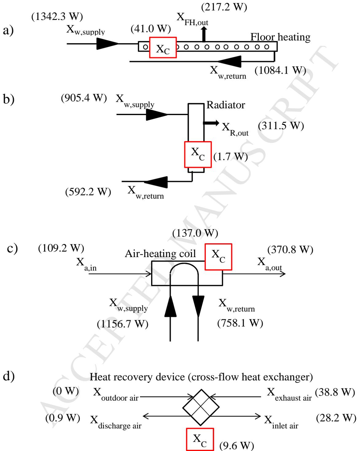
**Fig. 4.** Exergy input, output, and consumption in different system components: a) Floor (FH\_LoRes) b) Radiator (R\_45) c) Air-heating coil (WAH\_HR) d) Heat recovery device (0.5 ach, floor heating and radiator cases). Values in the parentheses indicate the exergy values.
