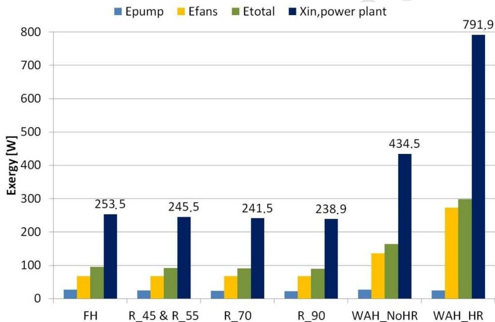
**Fig. 7.** Required exergy inputs to the pump, fans and to the power plant (four bars in each case indicate, from left to right, the exergy input to pump, to fans, their total, and the exergy input to the power plant)
