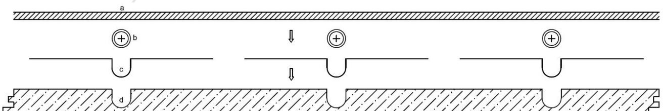
Fig. 2. a) Floor covering b) Pipe, 17x2.0 mm c) Heat distribution plate, 0.3 mm, d) Under-floor plate, 22 mm
