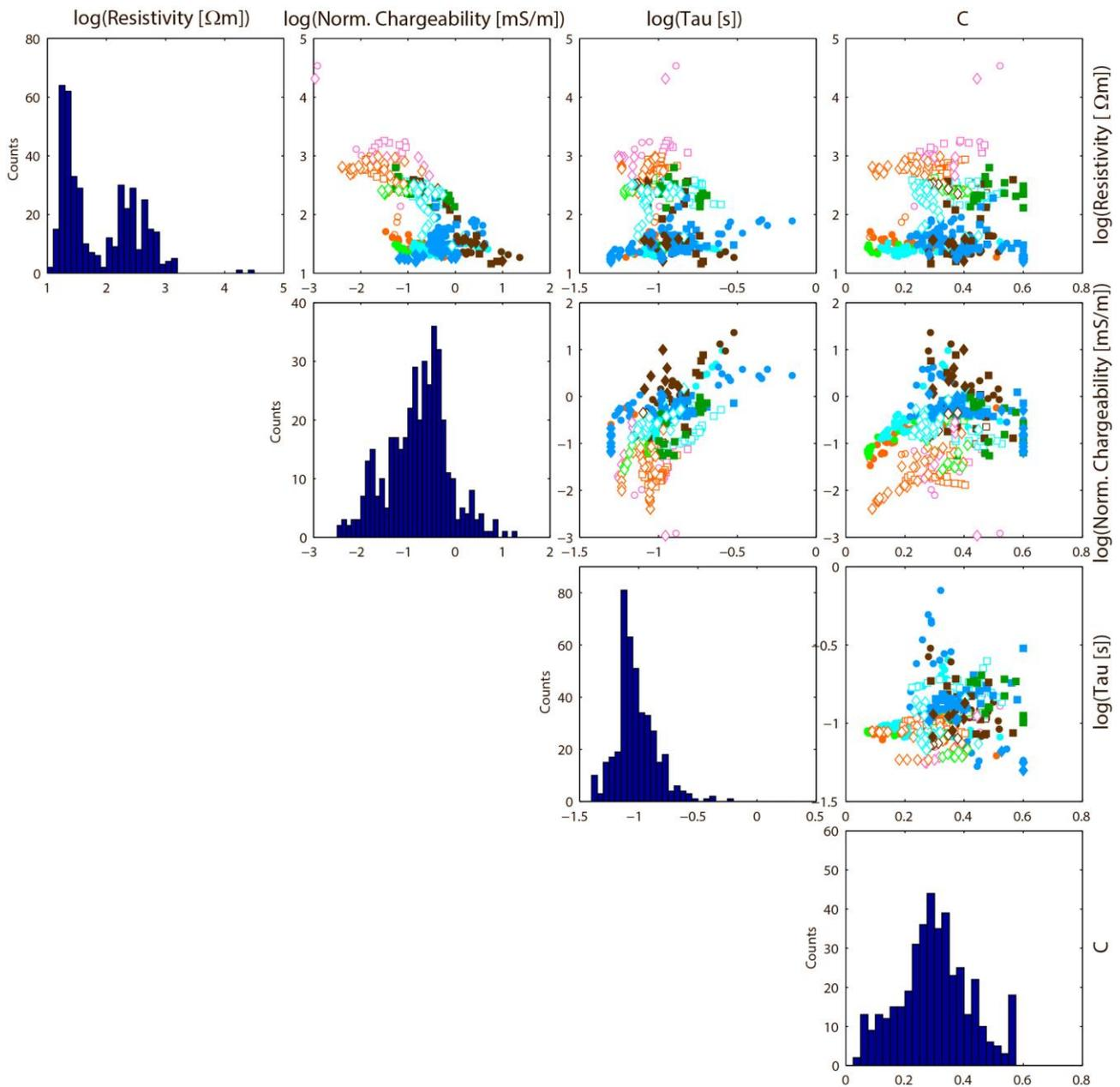
**Figure 2.** Histograms and cross plot of the Cole-Cole parameters from the three El-log drillings. The parameters are colour coded according to the geological log in Figure 1. An open plotting symbol indicates no or weak concentrations of contaminants, while a filled plotting symbol indicates high concentrations of contaminants. Data from B1, B3 and B5 are marked with a circle, square and a diamond, respectively.
