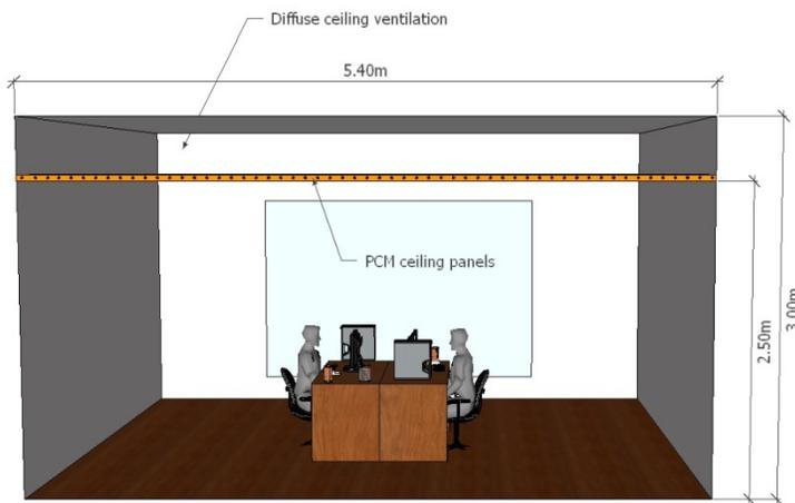
**Figure 1. Vertical cross-section of the simulated office room**
