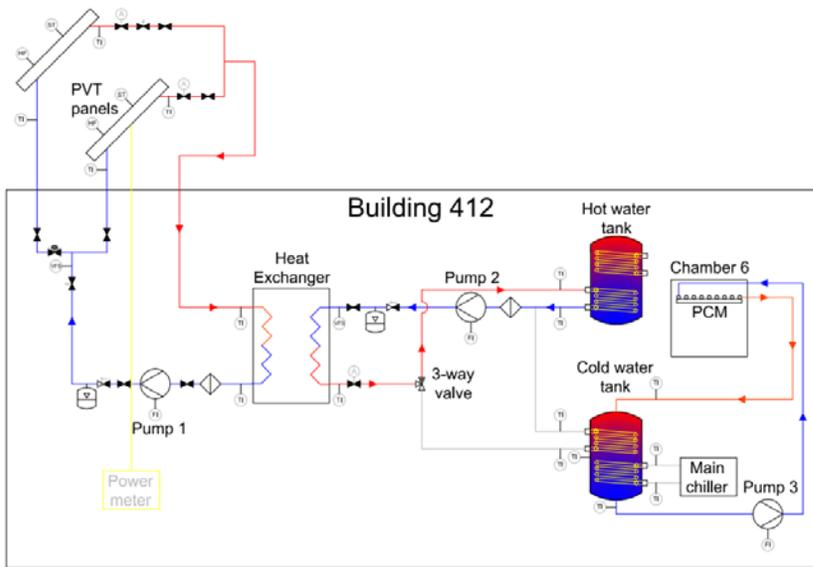
**Figure 2. Schematic drawing of the hydronic system**
