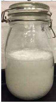
Figure 2. 1.3 kg PCM composite based on SAT in glass jar.
