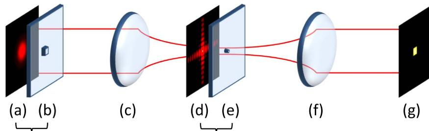
**Fig. 1.** Standard GPC setup consisting of an input phase mask (b), Fourier lenses (c) & (f) and a PCF (e). The input illumination (a), its Fourier transform, after applying the phase mask (d) and the imaged intensity (g) are also shown. (Not drawn to scale).
