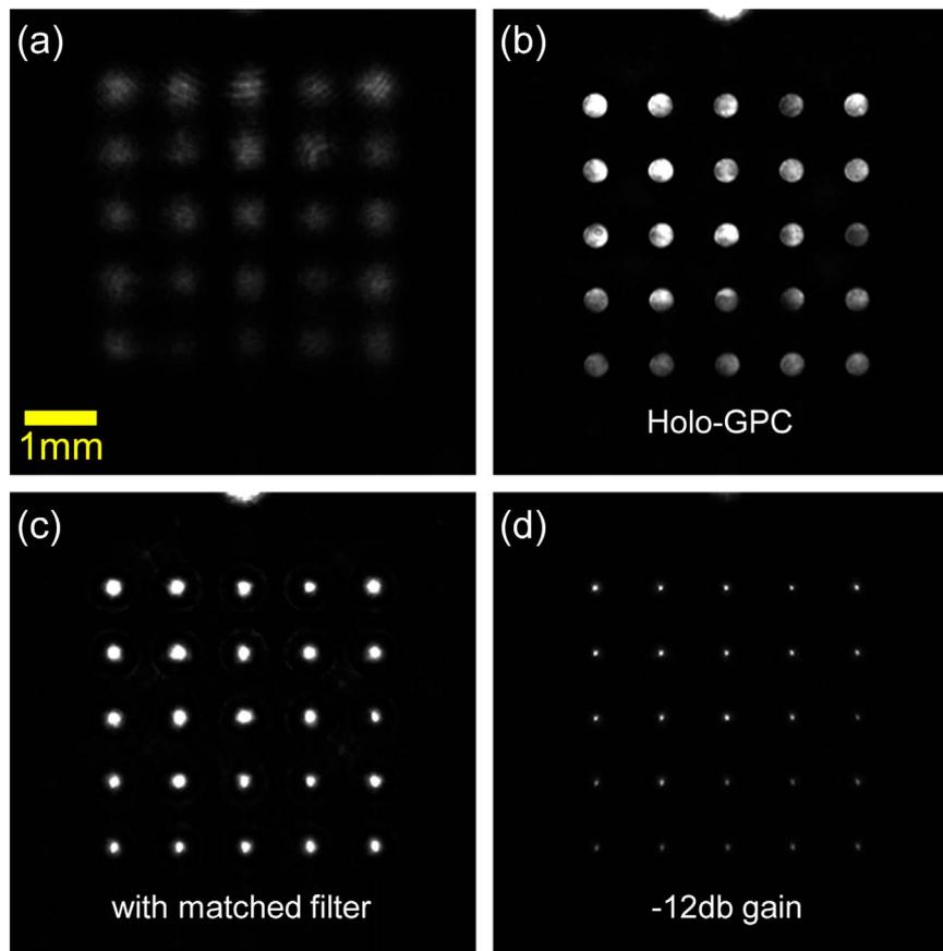
**Fig. 6.** A 5×5 holographically diffracted Gaussian spot array (a) shaped into circles via Holo-GPC (b), then converted into intense spikes (c) via matched filtering. To reduce the saturation (d), the camera gain had to be 12db lower.
