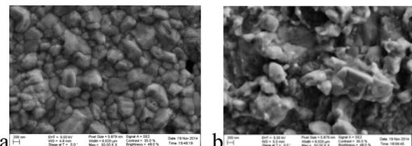
**Fig. 1** SEM images of annealed Cu-Sn-S films on Mo/SLG. **a**: deposited at 2.2 J/cm<sup>2</sup>, precursor ~1320 nm thick; **b**: deposited at 0.7 J/cm<sup>2</sup>, precursor ~4200 nm thick. Magnification 50k.
