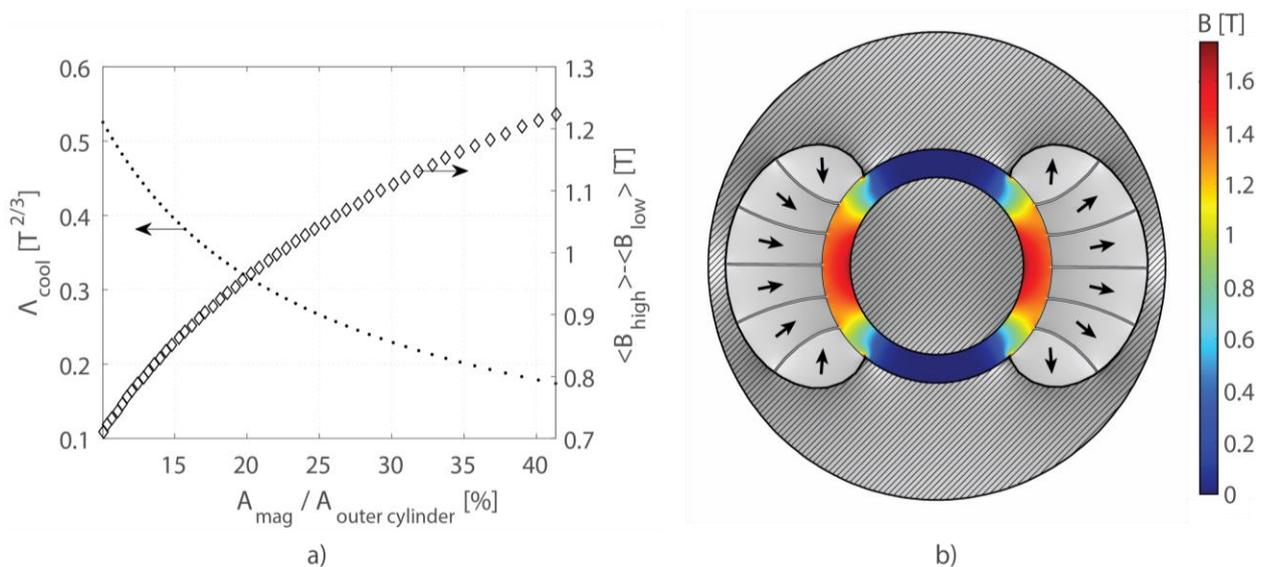
Figure 2: a) The  $\Lambda_{\text{cool}}$  and the difference in averaged field between the high and low field regions as function of the amount of permanent magnet material and b) the optimal magnet design for the case of  $A_{\text{mag}} / A_{\text{outer cylinder}} = 36\%$ .
