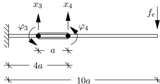
Figure 3. Beam with nodal displacement  $x_j$  and rotation  $\varphi_j$  and piezoelectric transducer pair.
