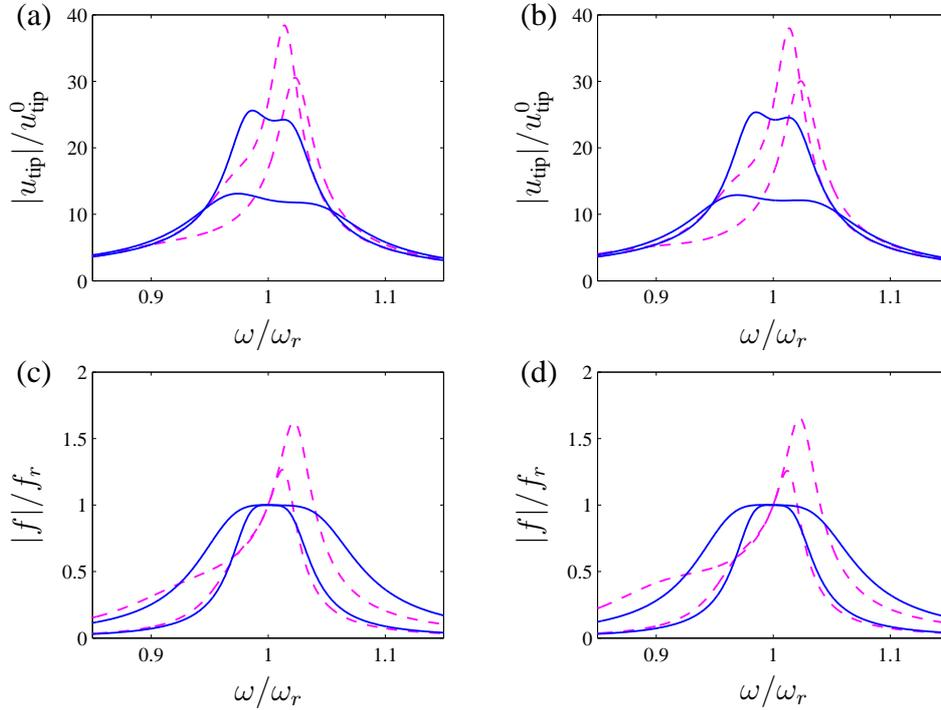
Figure 4. (a,b) Dynamic amplification and (c,d) force amplitude for (a,c) series and (b,d) parallel  $RL$  shunt circuit.
