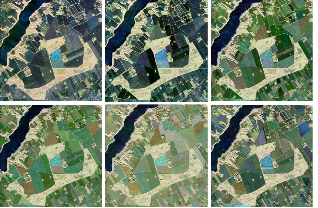
Fig. 1. RGB images of diagonal elements of the L-band data March, April, May (top row, left to right), June, July, August (bottom row, left to right).
