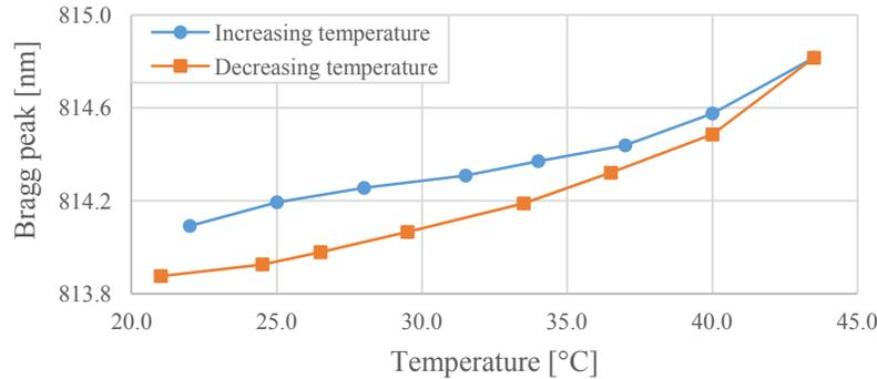
Figure 3. Temperature response of the embedded POFBG.
