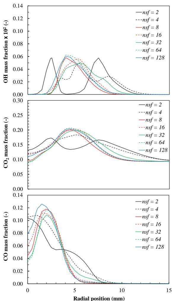
Figure 1: Comparisons of OH mass fraction, CO<sub>2</sub> mass fraction and CO mass fraction using different number of stochastic fields across the diffusion flame.
