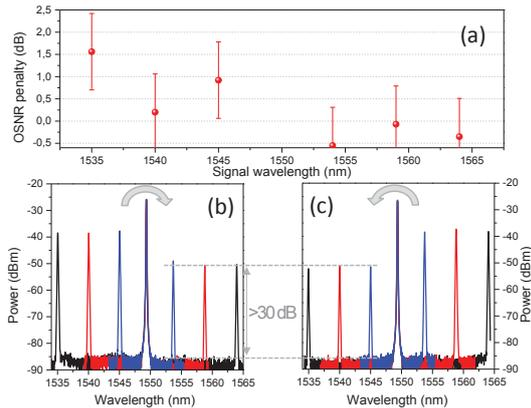
**Fig. 4:** (a) OSNR penalty as a function of the signal wavelength for a post-FEC BER of  $2 \times 10^{-2}$ ; (b) and (c) optical spectra at the waveguide output for signals on the short (b) and long (c) wavelength side of the pump. Idler OSNRs above 30 dB are shown for all the cases.
