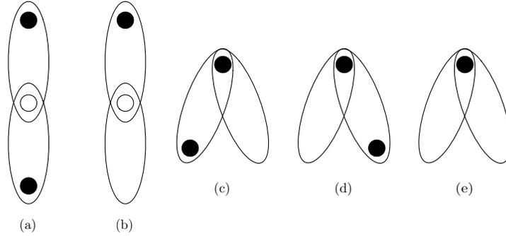
Figure 2: Five ways of merging clusters. The  $\bullet$  nodes are boundary nodes that remain boundary nodes in the merged cluster. The  $\circ$  nodes are boundary nodes that become internal (non-boundary) nodes in the merged cluster. Note that in the last four merges at least one of the merged clusters has a top boundary node but no bottom boundary node.
