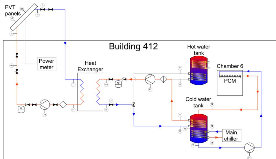
Figure 4: Schematic drawing of the hydraulic system
