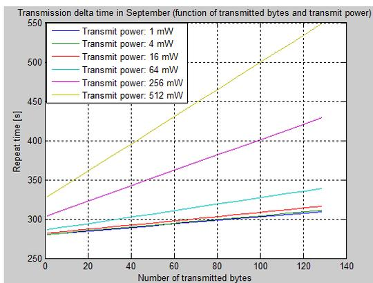
Fig. 8. The time between each transmission as a function of message length, transmit power and solar power available in september month (Denmark)
