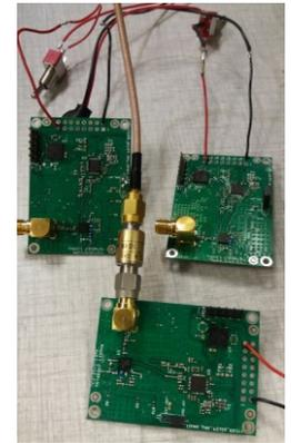
Fig. 2. Current consumption @3.1V for RF169MHz module with PA activated (leftmost) Hardware RF modules based on the wireless CC1125 device (rightmost).
