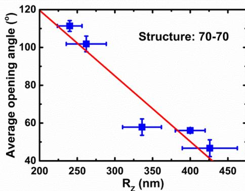
**Fig.4** Plot of the average opening angle of cones vs.  $R_Z$  for foils fabricated with 70-70 at  $T_C = 70^\circ$  C. The dashed red trend line is added to guide the eye. Error bars represent one standard deviation (n=4).
