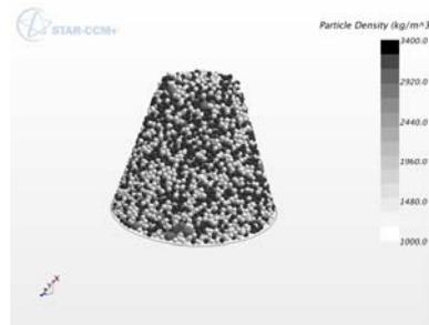
Figure 6. The initial condition for the numerical model. The three phases are water, cement, and mylonitic quartz diorite.
