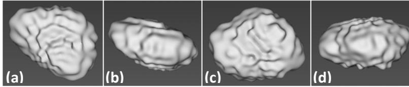
Figure 3. VRML images of particles based on the results from  $\mu$ CT scanning and SH analysis; (a), (b) two views of a mylonitic quartz diorite particle of VESD = 52  $\mu\text{m}$ ,  $L/T = 2.00$  and  $L/W = 1.38$ ; (c), (d) two views of a limestone particle of VESD = 52  $\mu\text{m}$ ,  $L/T = 1.82$  and  $L/W = 1.32$ . The number-weighted particle aspect ratios represents the mean values of the whole powder samples, as introduced above.
