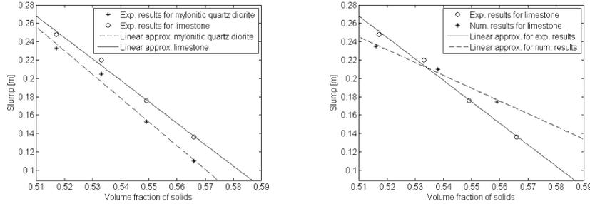
Figure 8. (left) Experimental slump results and linear approximation for the mylonitic quartz diorite and limestone based matrices at different volume fraction of solids when using  $\chi=0.35$ . (right) Experimental and numerical slump results and linear approximation for the limestone based matrices at different volume fraction of solids when using  $\chi=0.35$ .
