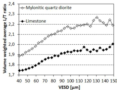
Figure 2. The volume weighted average  $L/T$  aspect ratio as a function of the size of the two fillers. Size given as volume equivalent sphere diameter (VESD). The average  $L/T$  for each size is based on a high enough number of particles to give converging  $L/T$  [5].
