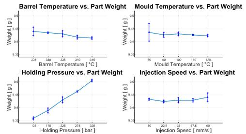
Figure 4: Main effect plots for injection parameters vs. part weight
