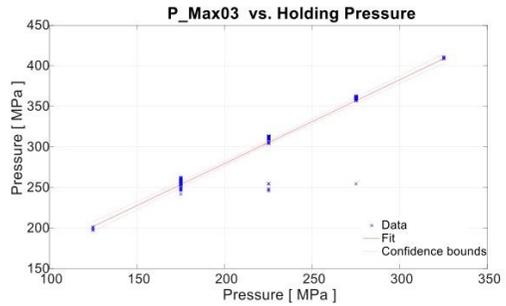
Figure 6: Regression analysis for holding pressure vs.  $P_{Max03}$
