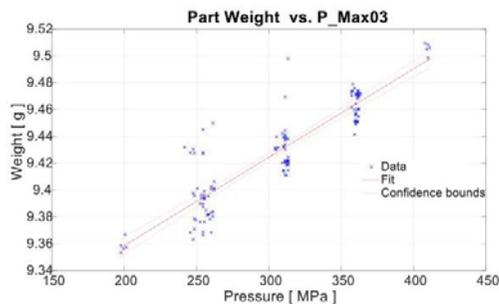
Figure 5: Regression analysis for part weight vs.  $P_{Max03}$
