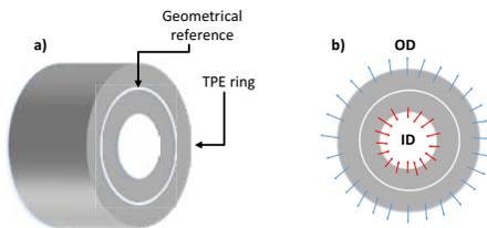
Figure 8: Illustration of TPE rubber ring geometrical reference. a) Side view indicating position of reference measurands to quantify ID and OD polymer behaviour; b) schematic top view of polymer shrinkage behaviour for OD and ID.
