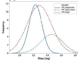
Figure 4: Comparison of part mass distribution for the different production batches. Data sheet batch (avg. value = 2, 28 mg ± 0,18 mg). High batch (avg. value = 2, 46 mg ± 0,16 mg). Improved batch (avg. value = 2, 23 mg ± 0,09 mg).
