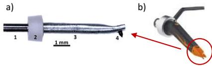
Figure 7: a) Assembled micro components [(1) Magnet (2) TPE suspension ring (3) Aluminium cantilever (4) Diamond tip]; b) Assembled high performance DJ cartridge.
