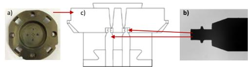
Figure 6: a) Mould plate containing 4 cavities; b) pin entering the cavity during injection moulding production of the suspension ring; c) mould cross section schematic view.
