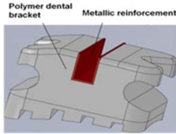
Figure 4: Polymer-metal micro insert moulded dental bracket.
