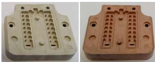
Figure 6: Injection moulded diplexer (left); plated diplexer (right).
