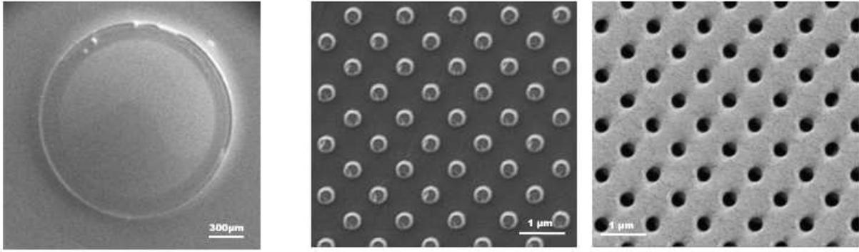
**Figure 1.** left: SEM of imprinted semi-sphere (top view,  $R=2.0\text{mm}$ ), center: SEM of imprinted semi-sphere presenting arrays of pillars on top of the sphere, right: SEM of injection molded polymer replica of the semi-sphere presenting arrays of holes on top of the sphere.
