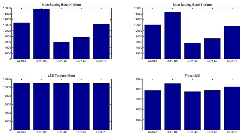
**Figure 3.** Variation in the extreme load under Design Load Case (DLC) 2.3 for different nacelle configurations: Geared – Conventional drivetrain with medium speed gearbox, Direct Drive King-pin (DDK)-100 overhanging generator concept with 100 % mass, DDK-40 - overhanging generator with 40% mass, DDK-50 - overhanging generator with 50% mass and DDK-75 - overhanging generator with 75% mass (as specified in table 2).
