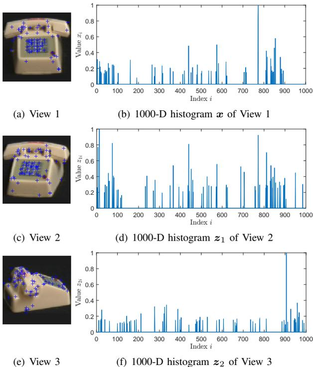
Fig. 1. SIFT-feature histograms of object 60 in the COIL-100 [31].
