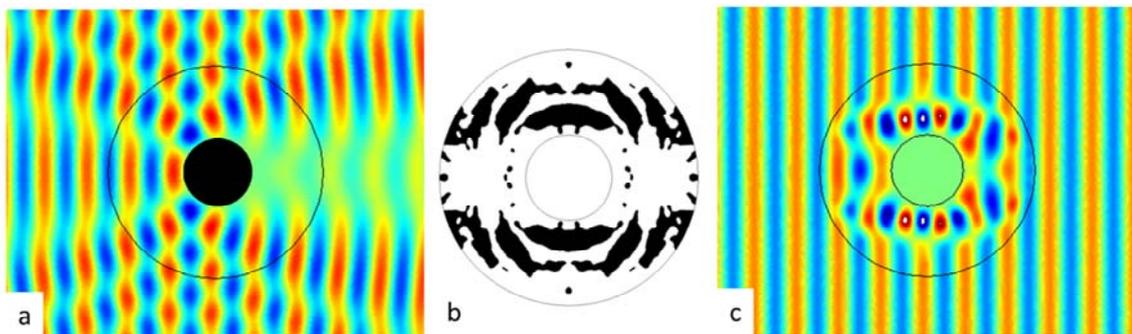
**Figure 3** Design of all-dielectric cloak using topology optimization. a) Scattering from hard cylinder. b) Topology optimization dielectric material distribution in cloaking domain (white: air, black: dielectric material,  $\epsilon_r=2$ ). c) Scattering from cloaked cylinder.
