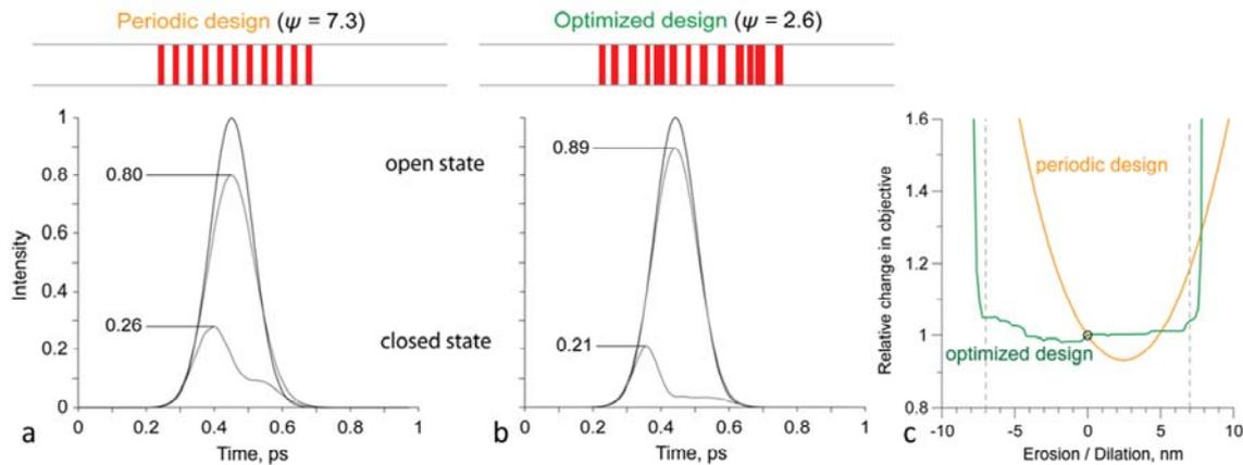
**Figure 2** a) Performance in open and closed states for simple Bragg-based non-linear photonic switch. b) Performance of optimized switch. c) Due to the robust optimization approach the optimized switch is less sensitive to under- or over-etching.
