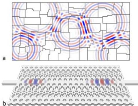
**Figure 1** a) Mesh partitioning for distribution of processes on parallel computer. b) Snap-shot of simulation results for 40M cell PhC slowlight waveguide test problem.
