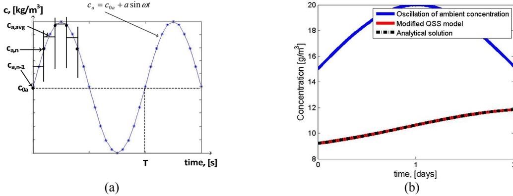
**FIGURE 2.** (a) Curve of ambient humidity which is divided into small time step intervals, (b) Comparison of the analytical solution and the modified QSS model. Here  $\omega$  is the oscillation's angular frequency (rad/s),  $a$  is the oscillation's amplitude, and  $c_{0a}$  is the initial offset amplitude ( $\text{kg}/\text{m}^3$ ).
