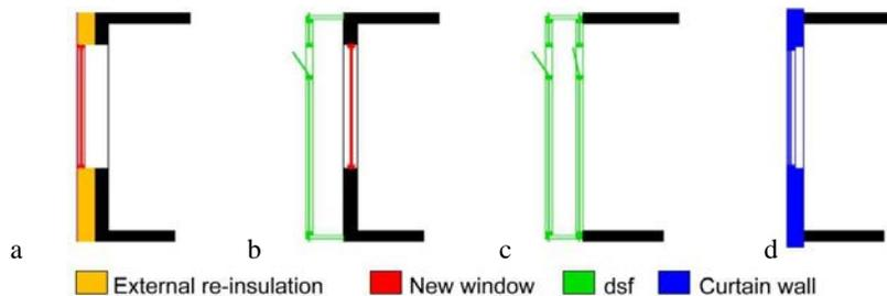
Figure 3 The renovation strategies: (a) External re-insulation (b) Double-skin façade (the external part) (c) Double-skin façade (d) Curtain wall.
