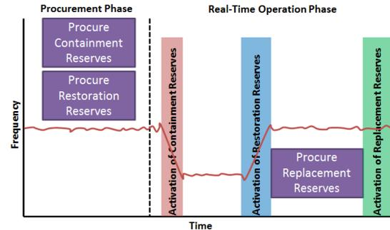
Fig. 2. Frequency management in Web of Cells
