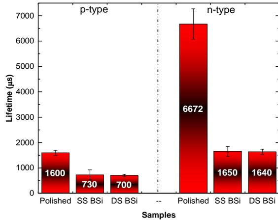
**Figure 5:** Comparative graph of average lifetime wafer mapping values with standard deviation for p- and n-type silicon samples with polished, single side nanostructured and double side nanostructured black silicon, passivated with ALD Al<sub>2</sub>O<sub>3</sub> 37 nm film. Legend: SS BSi - single side nanostructured black silicon, DS BSi - double side nanostructured black silicon
