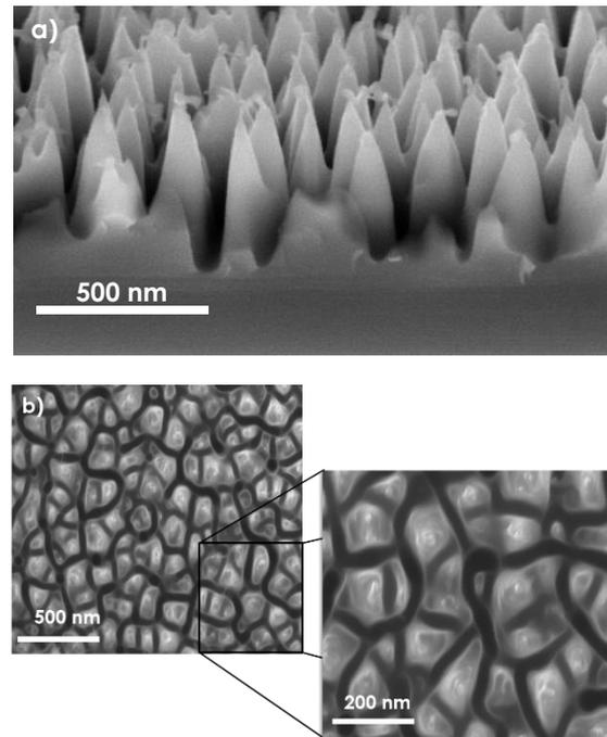
**Figure 3:** SEM image of the black silicon nano-structure topology processed with plasma assisted mask-less reactive ion etching: a) side view with scale 500 nm, b) top views with scale 500 nm and 200 nm
