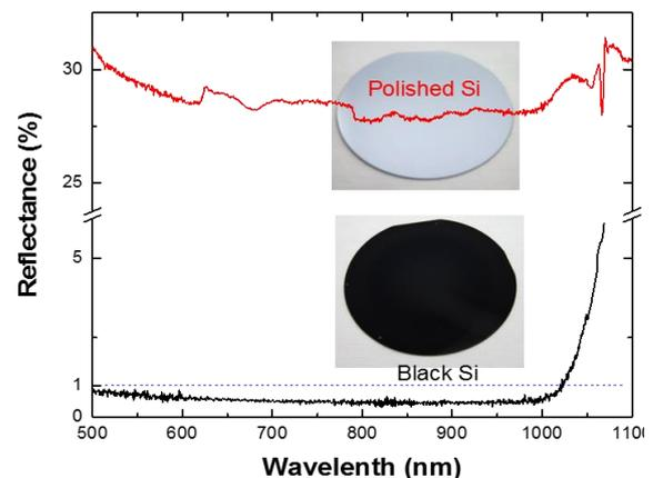
**Figure 4:** Experimental reflectance spectra of polished and black silicon without Al<sub>2</sub>O<sub>3</sub> coating
