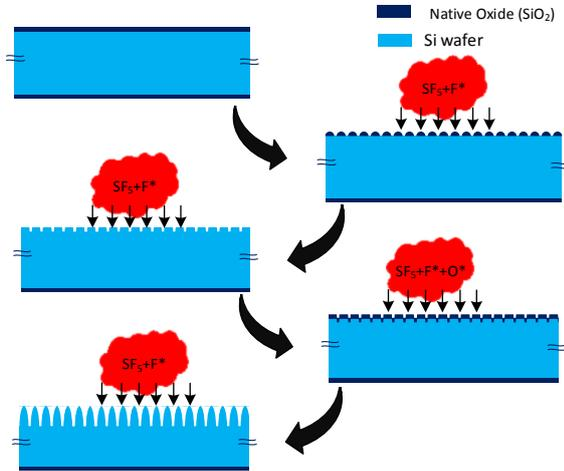
**Figure 2:** Schematic view of black silicon nanostructures formation
