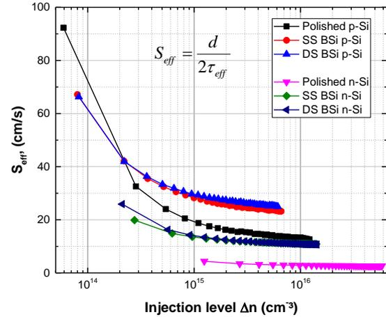
**Figure 7:** Surface recombination velocity dependencies on injection level
