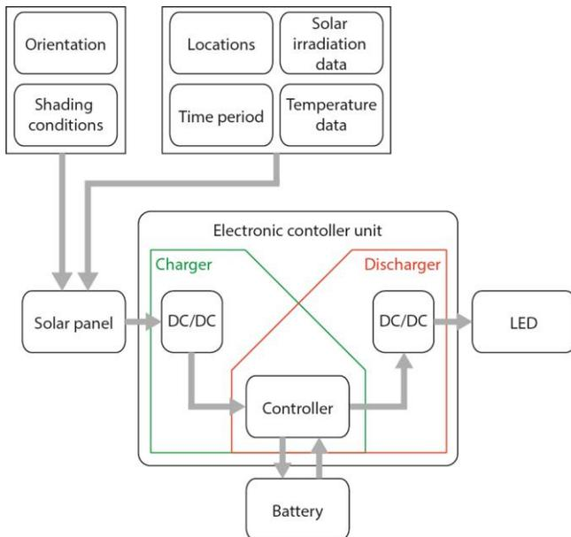
Fig. 4. Block diagram of L2L modelling tool.
