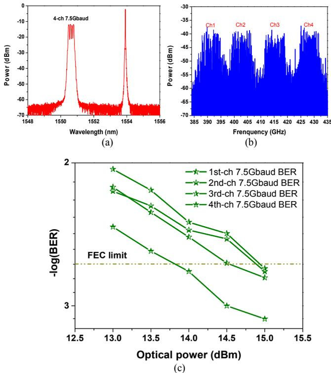
Fig. 4 (a) and (b) are optical spectrum and electrical spectrum of the 4-channel THz signals, respectively. (c) BER performance of four THz channels after 50 cm wireless transmission.
