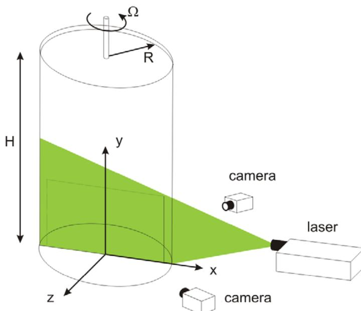
**Figure 1:** Sketch of setup for stereoscopic PIV measurement
