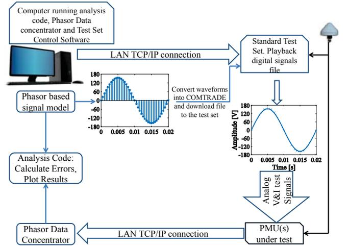
Fig. 2: Block Diagram of the Test Platform
