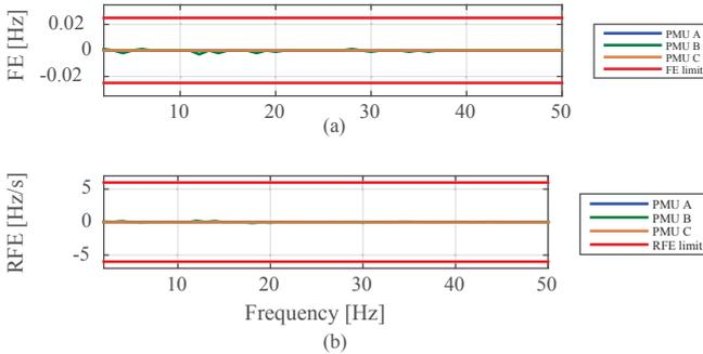
Fig. 10: Harmonic rejection Test: a) Frequency Error; b) ROCOF Error
