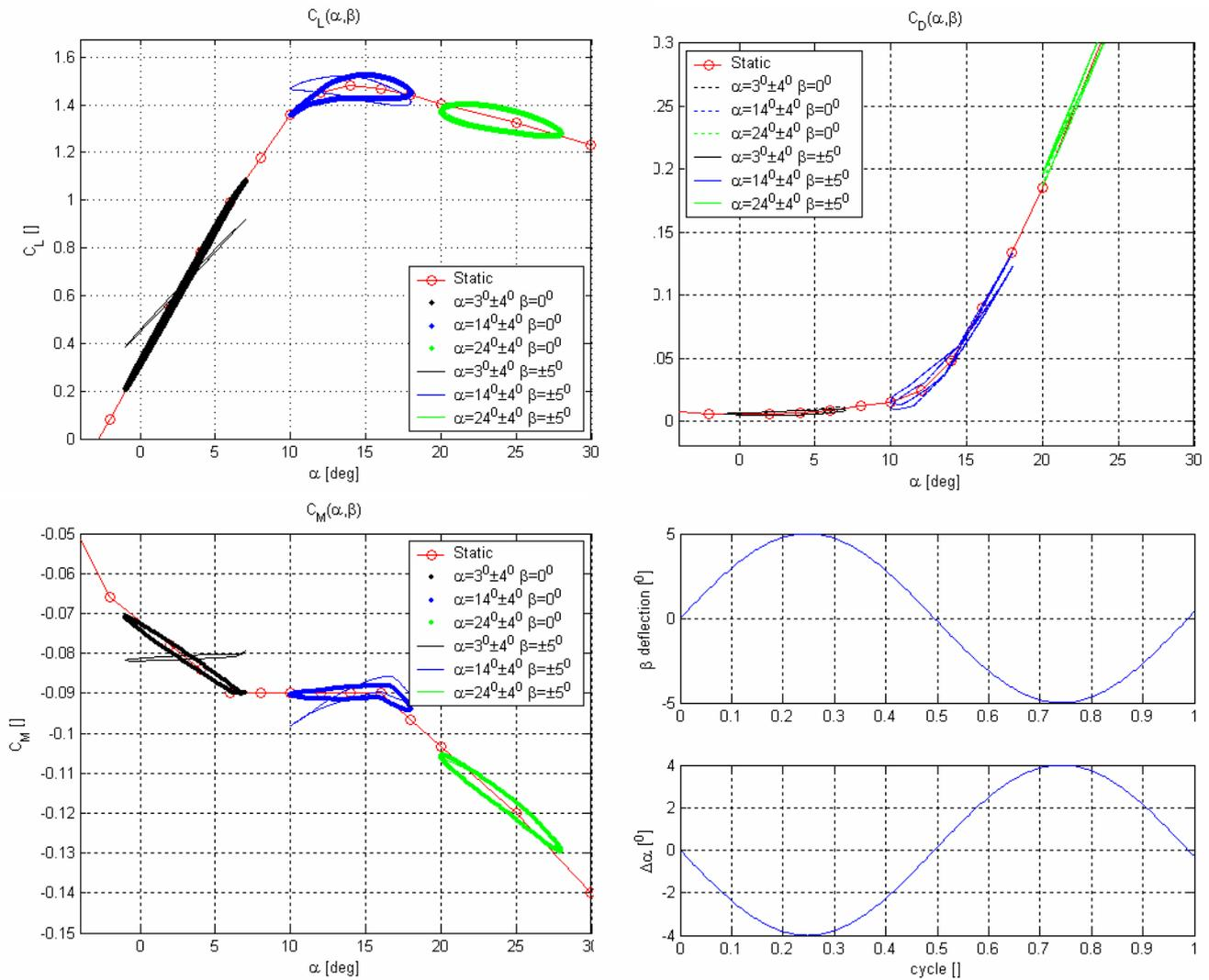
Figure 4. Response of  $C_L$ (upper left),  $C_D$ (upper right) and  $C_M$ (lower left) to oscillatory pitching motion without the use of DTEG deflection and with use of DTEG deflection. The results are given by the suggested model using the DTEG measurements of static lift, drag and moment coefficients on a B1-18 profile as input. Reduced frequency is  $k=\omega c/(2U_0)=0.1$ .  $\Delta\alpha=4^\circ \Delta\beta=5^\circ$
