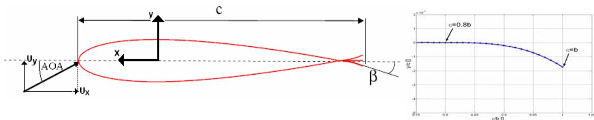
Figure 1 Left: Airfoil equipped with a DTEG.
