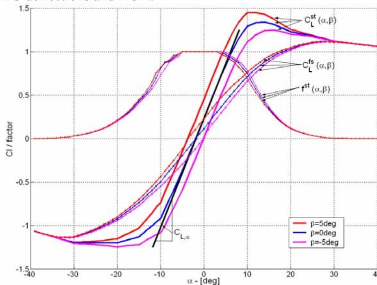
Figure 2  $C_L^{st}$ ,  $C_L^{fs}$  and  $f^{st}$  for DTEG deflection of  $\beta = -5^0, 0^0, 5^0$  at AOA from +/-  $40^0$ .
