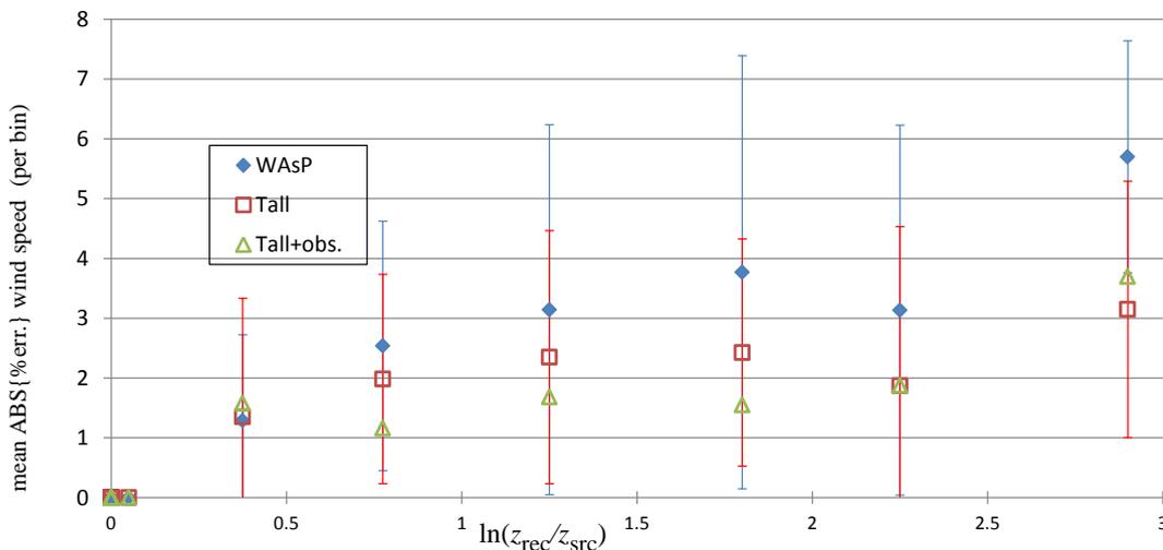
**Figure 4.** Mean of absolute error in wind speed extrapolation per relative extrapolation bin in  $\ln(z_{rec}/z_{src})$ , also using measured flux statistics (yellow triangles) instead of the ‘default tall’ parameters (red squares).
