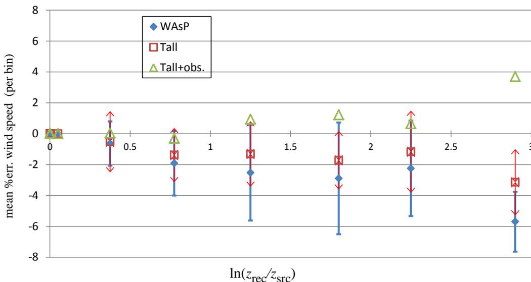
**Figure 5.** Mean error in wind speed extrapolation per relative extrapolation bin in  $\ln(z_{rec}/z_{src})$ , also using measured flux statistics (yellow triangles) instead of the ‘default tall’ parameters (red squares).
