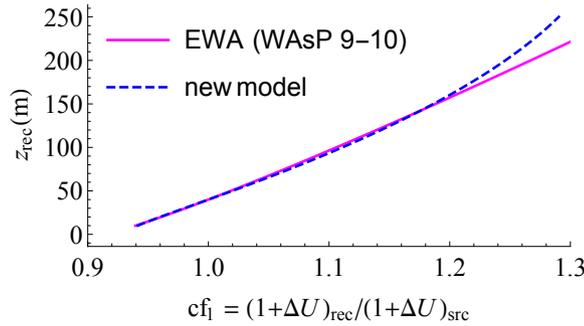
**Figure 1.** Profile of mean wind speed correction factor (dimensionless wind profile)  $cf_1(z)$  for source and target sites, via EWA (magenta) and new tall (blue/dashed) model (17). Observation height is  $z_{src} = 40 \text{ m}$  and corresponding roughness length is  $z_{0,src} = 3 \text{ cm}$ ; here with typical stability statistics  $\{\sigma_{\pm}, n_+, h_{eff}\}$  and suggested EWA parameters  $\{H_{off}, H_{rms}\}$ .
