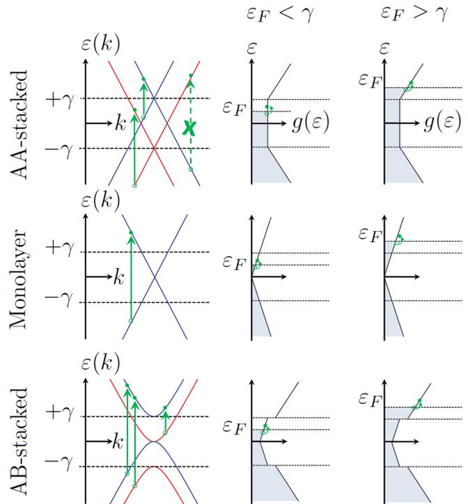
FIG. 2. Schematic electronic band structures  $\varepsilon(k)$  (left column) and electronic density of states  $g(\varepsilon)$  (middle and right columns) of AA-stacked, monolayer graphene, and AB-stacked bilayer graphene. The arrows indicate possible and prohibited (dashed style arrow) single-particle interband transitions (vertical transitions) as well as intraband plasmonic excitations near the Fermi level  $\varepsilon_F$ .
