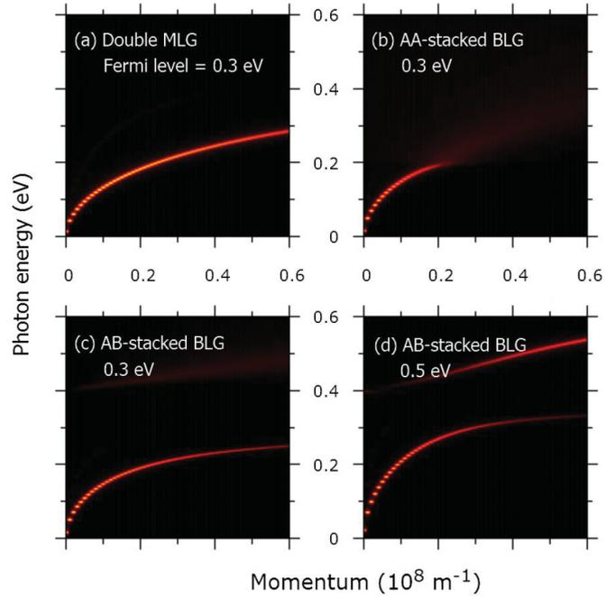
FIG. 4. The extracted plasmonic dispersion band diagrams at  $\epsilon_F = 0.3 \text{ eV}$  of (a) double MLG nanodisks, (b) AA-stacked BLG nanodisks, (c) AB-stacked nanodisks, and (d) AB-stacked nanodisks for  $\epsilon_F = 0.5 \text{ eV}$ .
