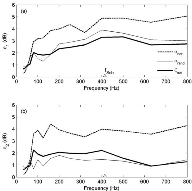
FIG. 4. Errors averaged over the receiver positions as a function of frequency in the proportionate room for a non-uniform absorption configuration. (a)  $e_1$ ; (b)  $e_2$ .  $\triangle$  indicates the Schroeder frequency.
