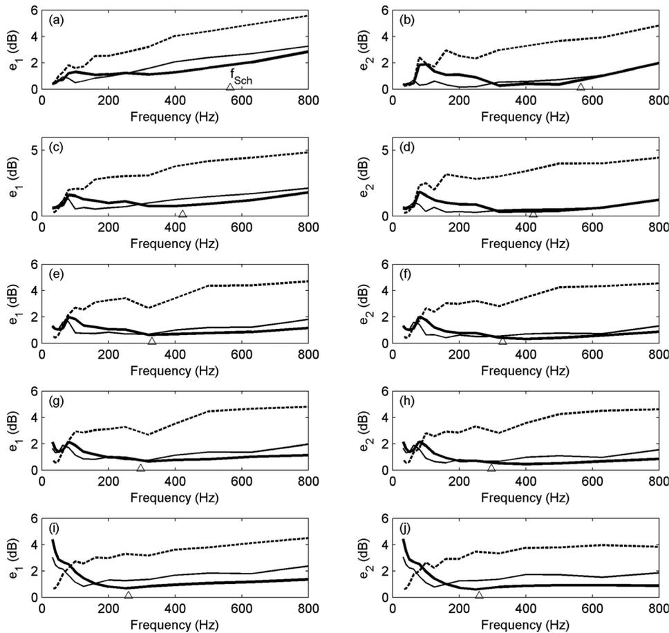
FIG. 1. Errors averaged over the receiver positions as a function of frequency in the proportionate room. (a), (c), (e), (g), and (i)  $e_1$ ; (b), (d), (f), (h), and (j)  $e_2$ . (a) and (b) BC1; (c) and (d) BC2; (e) and (f) BC3; (g) and (h) BC4; (i) and (j) BC5. —  $\alpha_{\text{nor}}$ ; —  $\alpha_{\text{rand}}$ ; and —  $\zeta_{\text{nor}}$ .  $\triangle$  indicates the Schroeder frequency.
