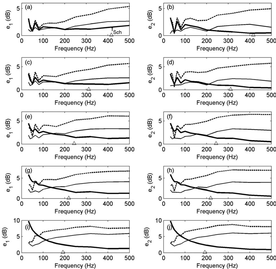
FIG. 6. Errors averaged over the receiver positions as a function of frequency in the disproportionate room. (a), (c), (e), (g), and (i)  $e_1$ ; (b), (d), (f), (h), and (j)  $e_2$ . (a) and (b) BC1; (c) and (d) BC2; (e) and (f) BC3; (g) and (h) BC4; (i) and (j) BC5. —,  $\alpha_{\text{nor}}$ ; —,  $\alpha_{\text{rand}}$ ; - · - ·,  $\zeta_{\text{nor}}$ .  $\triangle$  indicates the Schroeder frequency.
