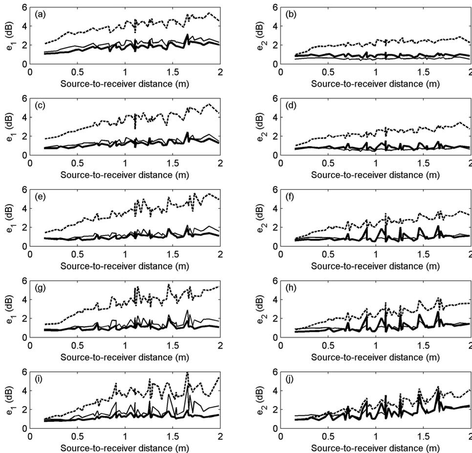
FIG. 2. Errors averaged over the frequency as a function of the source-to-receiver distance in the proportionate room. (a), (c), (e), (g), and (i)  $e_1$ ; (b), (d), (f), (h), and (j)  $e_2$ . (a) and (b) BC1; (c) and (d) BC2; (e) and (f) BC3; (g) and (h) BC4; (i) and (j) BC5. —,  $\alpha_{\text{nor}}$ ; —,  $\alpha_{\text{rand}}$ ; —,  $\alpha_{\text{nor}}^z$ .
