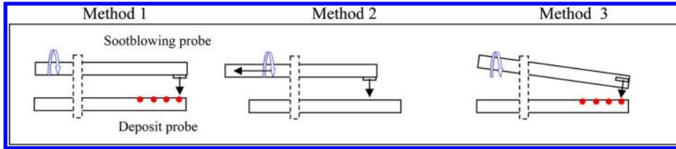
Figure 4. Experimental methods applied for artificial sootblowing.
