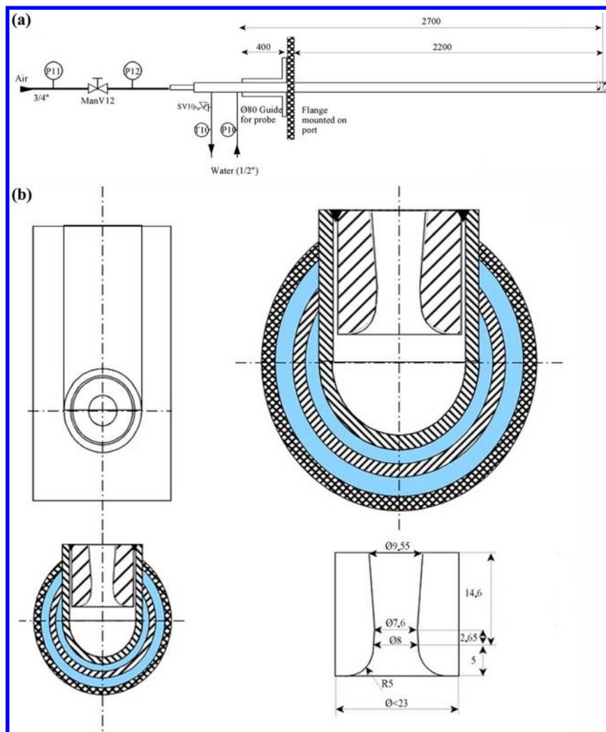
**Figure 2.** (a) Schematic of sootblowing probe with water and air flow description: P10, P11, and P12 are pressure gauges for air, P10 is a pressure gauge for water (to act as a cooling medium), and T10 is temperature indicator. (b) Detailed drawings of the sootblowing nozzle.
