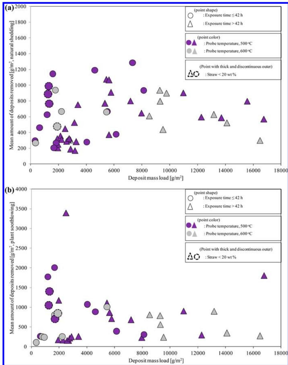
**Figure 8.** Impact of deposit mass load on (a) the mean amount of deposits removed naturally and (b) the mean amount of deposits removed by plant sootblowing. Data points are from tests 1–5. The particular point shape represents the exposure time, and the color represents the probe surface temperature, whereas points (larger in size) with thick and discontinuous edges are representative of straw share in wood.
