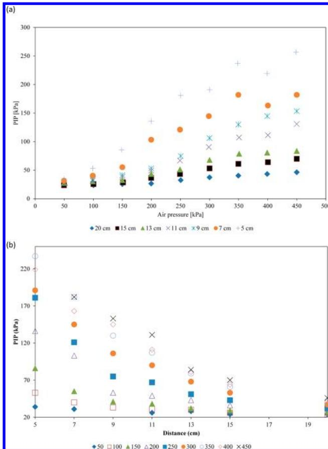
**Figure 3.** Measured peak impact pressure (PIP) as a function of (a) applied air pressure at various downstream distances from the nozzle exit to the deposit probe at room temperature and (b) distance from the nozzle exit to the deposit probe at various pressures at room temperature.
