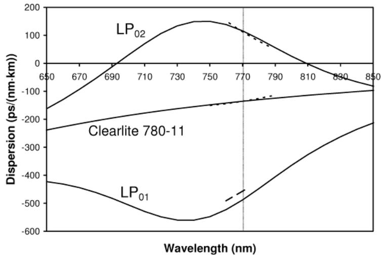
Fig. 1. Dispersion curves as calculated from the refractive index profile of the fiber preform of LP<sub>02</sub> HOM and LP<sub>01</sub> fundamental mode. Also shown is the calculated dispersion of the single mode fiber ClearLite 780-11. Dotted curves are corresponding dispersion curves measured with a white light interferometer.
