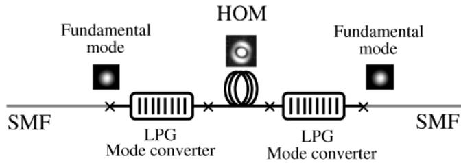
Fig. 2. Solid-silica fiber module for femtosecond pulse delivery.
