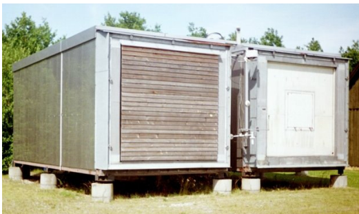
FIG. 1: Picture of the test cells at DTU. Only the test cell on the left is used for the experiments presented in the paper.
