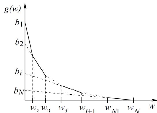
**Fig. 1** The scheme of multi-linear softening curve.
