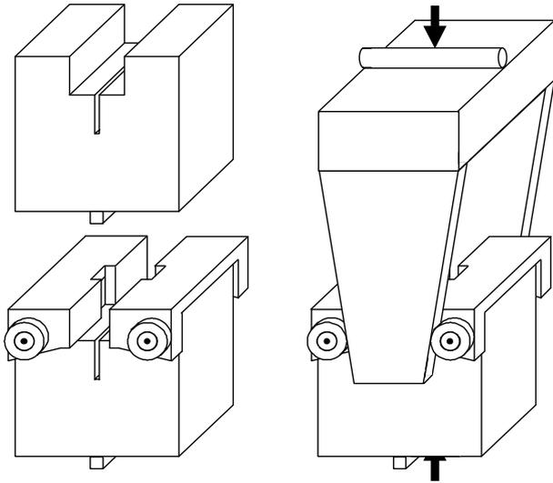
Fig. 4 Schematic showing of experimental WST test setup.
