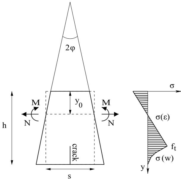
Fig. 2 The hinge model and assumed stress distribution.
