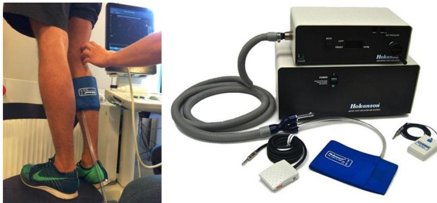
Figure 2: (left) The experimental set-up with ultrasound examination of the right popliteal vein while the right leg is unsupported and the lower leg is compressed with (right) a cuff compression-decompression system.
