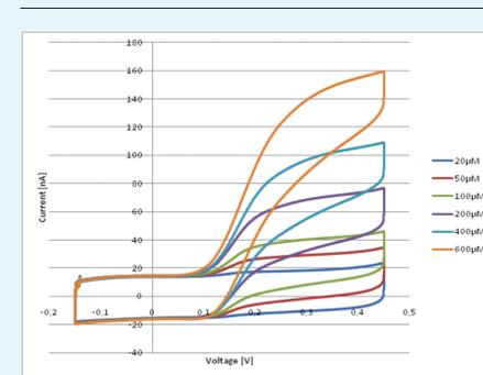
Figure 4: Cyclic voltammograms showing the oxidation of dopamine on a PEDOT electrode. Dopamine was diluted in PBS buffer. Scan rate: 10 mV/s, electrode dimensions:  $50 \mu\text{m} \times 1500 \mu\text{m}$ . The large hysteresis is due to the high capacitance of PEDOT
