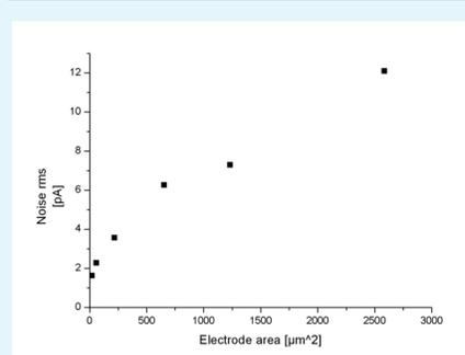
Figure 5: Noise versus electrode area. The noise was calculated as the root mean square noise of a current trace with the electrode being exposed to phosphate buffer.
