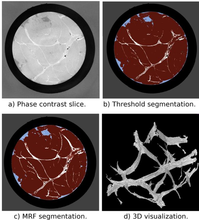
**Figure:** In a) a single slice from the phase contrast tomogram is shown, b) illustrates the results from a conventional threshold segmentation, c) shows the results from the anisotropic MRF segmentation and d) shows a 3D visualization of part of the segmented connective tissue.
