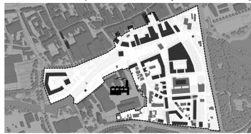
Fig. 4: Investigated area (light coloured) with old building stock (grey), new developments (black) and waste heat sources (icon).
