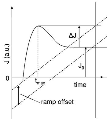
FIG. 4. Scheme of the dark CELIV measurement. The linear increasing ramps are shown by the dashed lines. For calculation of the mobility the distance between  $t_{\max}$  and the intersection of the shifted ramp with the time axis is used for mobility calculation.
