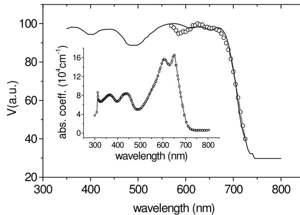
FIG. 9. Normalized photovoltage spectra of PBDT-DTBTff. Full line - theory fitted to the experimental points with the parameters:  $w = 40$  nm,  $d = 90$  nm,  $L = 12$  nm. The inset shows the spectral dependence of absorption coefficient.
