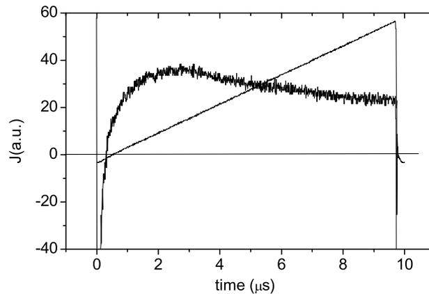
FIG. 7. CELIV curve of PBDT-DTBTff polymer. The straight line shows the shifted ramp used for mobility calculation.
