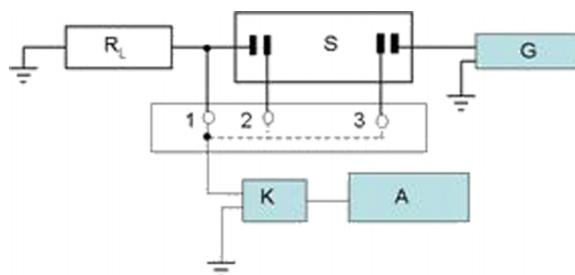
FIG. 2. Conductivity measurement: Current is calculated from the voltage drop on the resistor  $R_L$  at point 1, the voltage on the sample is measured at points 2 and 3. K is the electrometer, A is the narrow band amplifier, G is the generator of the alternating signal.
