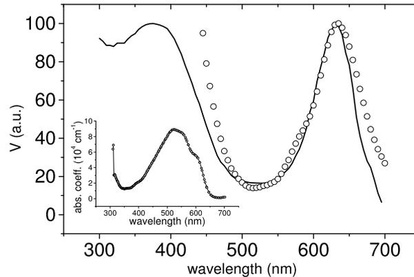
FIG. 10. Normalized photovoltage spectra of P3HT. Full line - theory fitted to the experimental points with the parameters:  $w = 20$  nm,  $d = 310$  nm,  $L = 6$  nm. The inset shows the spectral dependence of absorption coefficient.
