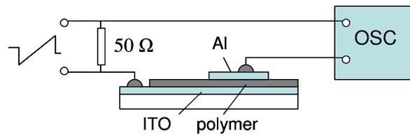
FIG. 3. Experimental set-up for the CELIV measurement.
