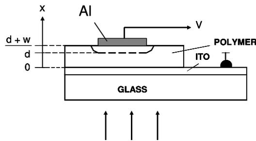
FIG. 5. Arrangement of the SPV measurement:  $w$  is the thickness of the space charge region under the Al electrode,  $d$  is the thickness of the neutral bulk where diffusion of the photogenerated excitons takes place.
